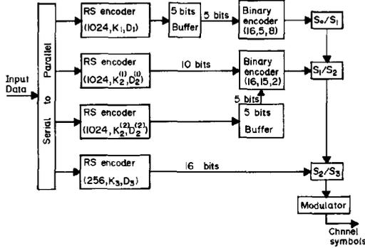
Fig. 6. Encoding scheme for Example 3.
