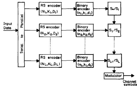
Fig. 1. Basic encoding scheme.
