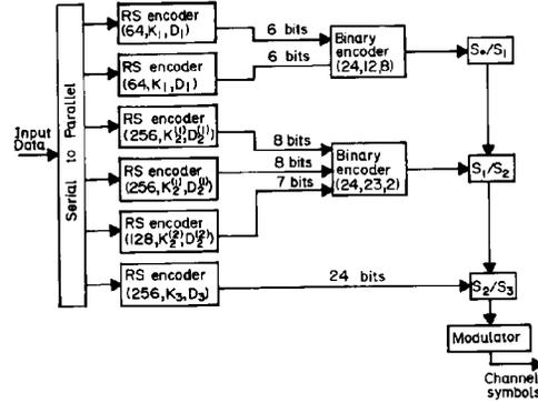
Fig. 4. Modified encoding scheme for Example 1.
