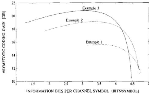
Fig. 7. Maximum obtainable coding gain for various values of  $R_{\text{eff}}$ .
