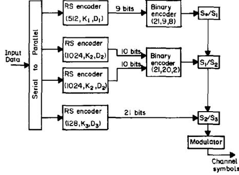
Fig. 5. Encoding scheme for Example 2.
