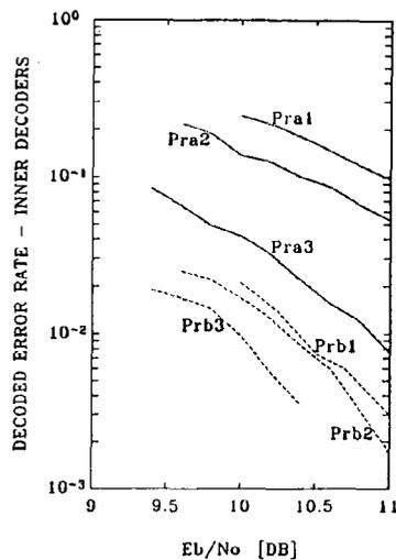
Fig. 8. Results of a computer simulation for outputs error rates of the inner decoders of Examples 1-3.
