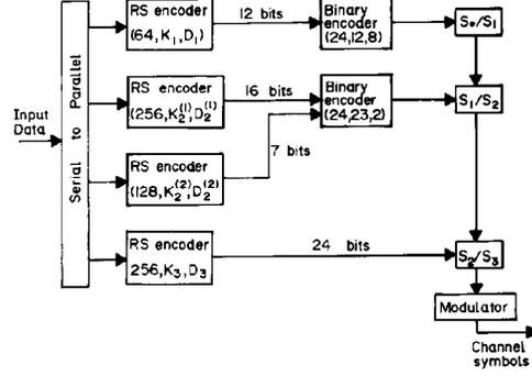
Fig. 3. Encoding scheme for Example 1.
